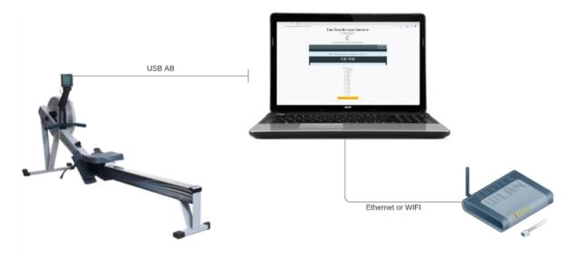
The required USB A/B cables are plugged into the rowing machine with the "B"-side (see image).
